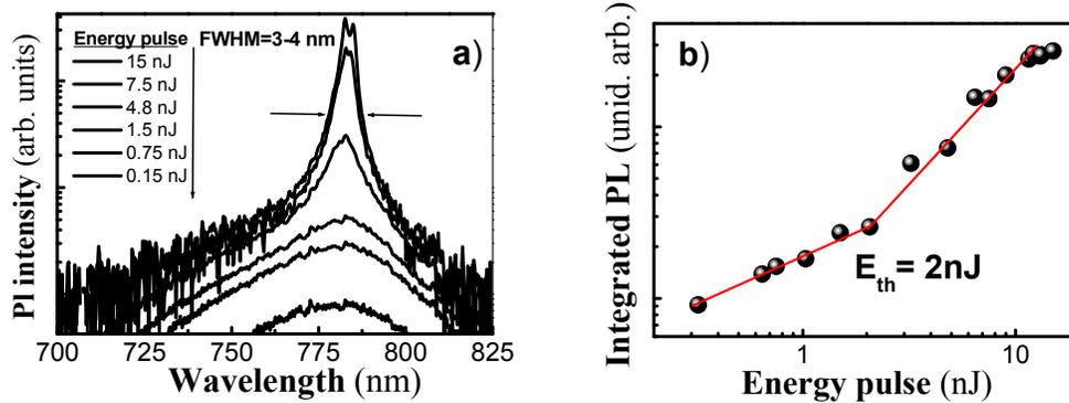
Fig. 2. a) PL spectra at the output edge of the waveguide for different excitation fluencies. b) Integrated PL as a function of the energy pulse. Narrowing of spectrum and superlinear increase of the integrated intensity indicates the generation of stimulated emission.
