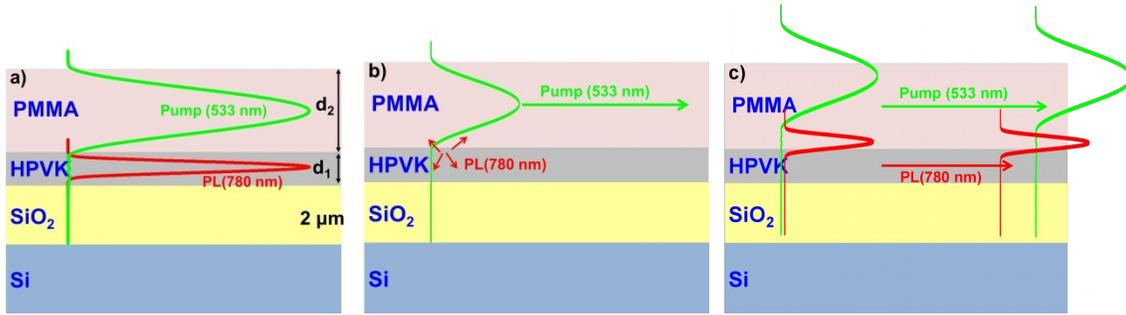
Fig. 1. a) Structure of the sample. b) Excitation beam at 533 nm is propagated along the PMMA layer and excites the semiconductor with the evanescent field. c) Low attenuation of the excitation beam in the PMMA allows the generation of PL along the whole length of the waveguide, which is propagated through the modes confined in the HPVK.
