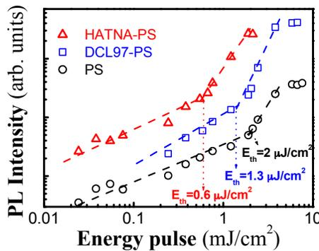
Fig. 3. PL intensity of HPVK layers (black), and HPVK layers incorporating DLC97 (blue) and HATNA (red) organic additives as a function of the energy pulse. Threshold of stimulated emission clearly decreases with the passivation of the organic compounds.
